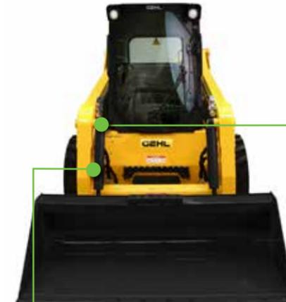
● OVER-THE-TIRE design provides wider access and improved visibility. *On the R220 and R260*
