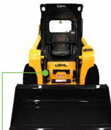
● BETWEEN-THE-TIRE design keeps machine length short and compact. *On the R190*
