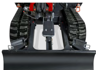
Retracted undercarriage : 980 mm
