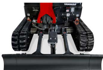
Extended undercarriage: 1320 mm
