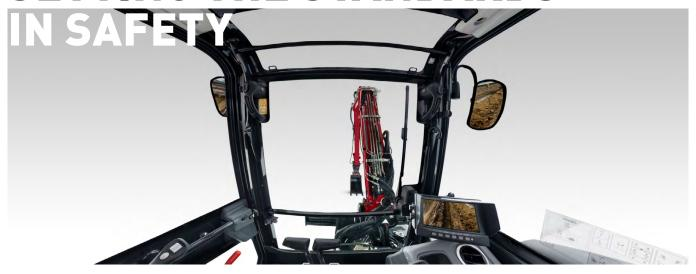
The SV60-6B cab has been designed to meet ROPS (Roll-Over Protective Structure) certification, as well as FOPS (Falling Object Protective Structure) level 1. The cab can be fitted with FOPS level 2 protection (front and top guard) as an optional extra.
