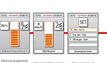
Electrical proportional adjustment of the hydraulic performance of the 3rd and 4th circuits.
