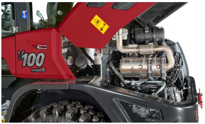
The large opening offered by the engine hood allows an easy access to all main service items, for an easy and fast maintenance. This contributes to reduce the total cost of ownership (TCO) of the machine. Daily tasks can be performed from ground level to save time.
