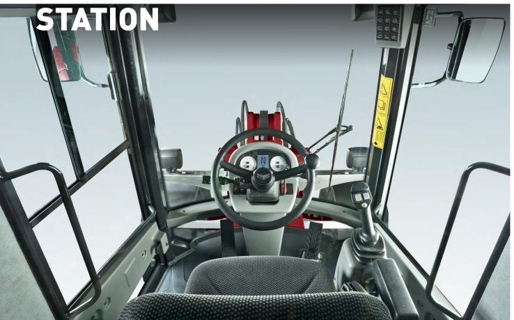
Designed with driver comfort and productivity in mind. The case feature ROPS and optional FOPS and noise and vibration damping - approved.
