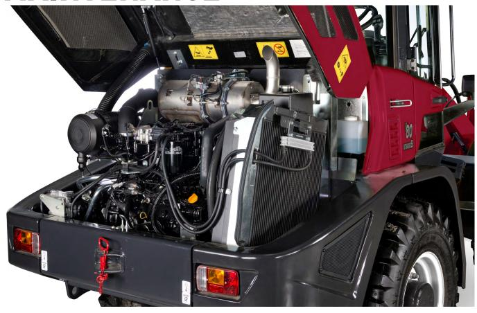
The large opening offered by the engine hood allows an easy access to all main service items, for an easy and fast maintenance. This contributes to reduce the total cost of ownership (TCO) of the machine. Daily tasks can be performed from ground level to save time.
