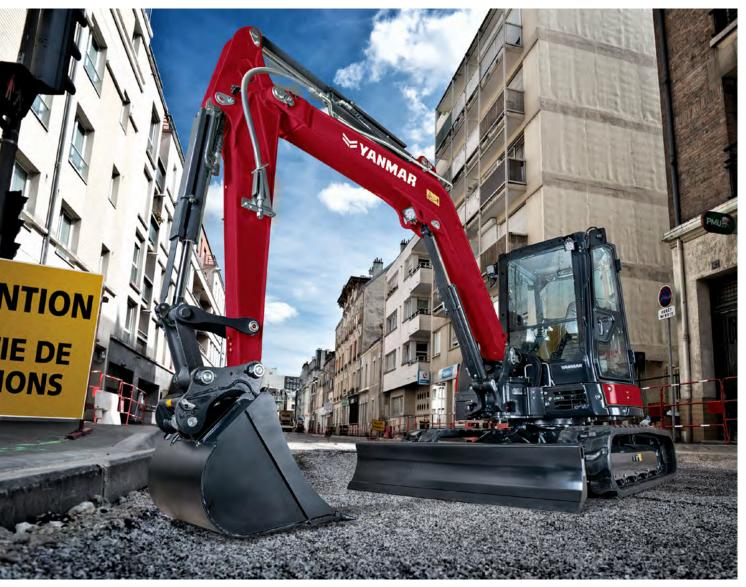
The Vi057-6B benefits from an improved powerful engine with Diesel Particulate Filter, the hydraulic pumps (+ 14 %) and a new control valve improve the cycle-times by more than 10 %.
